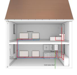
2) Conventional boiler: (also known as heat-only boiler) requires a hot water tank or cylinder, in which hot water can be stored for later use.
